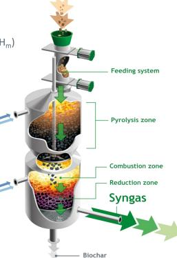
NOTAR® Technology is the integration of three independently designed and controlled reactors in a **compact** way. The technology produces clean syngas from different types of **biomass**.
